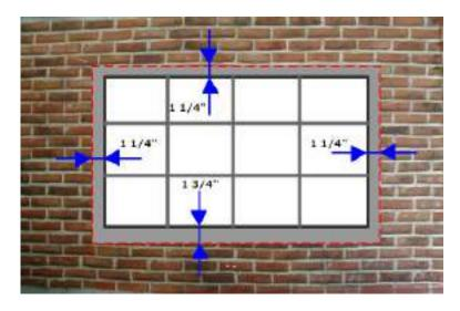
Install the extensions in the spaces left between the brick/stone and the openings, and install the mouldings on top.
