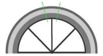
3. Glue the keystone, and the two half arches in place. Use FLEXOCOAT in the joins.
