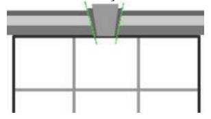
2. Place the half headers on the window, mark the cut lines, cut the trims. Take into account the angles on the sides of the keystone.
